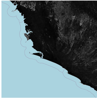
Figure 1: A map showing the difference in terrain ruggedness index (TRI) as calculated by the gdaldem tri command between GDAL versions 3.2 and 3.3. The difference would ideally be zero (all black) but includes pixels as different as 372 metres.
